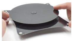
15. Check the fit by temporarily placing the spacers between the boards. The disks should have only about 2-3 mm of separation, and there should only be a very small gap between the ends of the spindles. Check there is greater than 0.5 mm between the charge collectors and the disk (a larger gap is fine). The charge collectors must not contact the disk.
