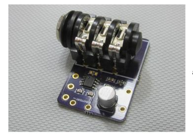
The ¼" Amplify Me kit is a LM386-based audio amplifier that is great for hobby-level audio projects, instruments, and radios!
