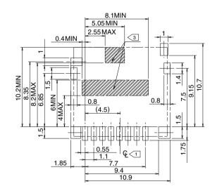
Note 1 $\mathcal{Q}$  indicates the center line of the microSD card slot. 2
