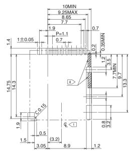
Note 1 4 indicates the center line of the microSD card slot.
