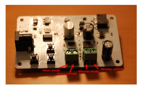
I would recommend using heat shrink to cover the wires. This offers protection against the high voltage and prevents the wires accidentally shorting to each other.
