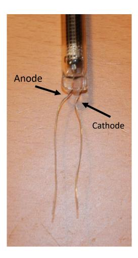
The anode and cathode need to be connected to these pins on the board:
