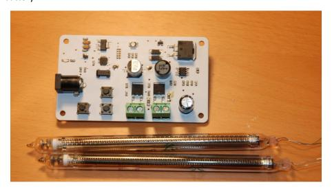
To power the PCB you will need a 12v 1A power supply with a 2.1mm DC jack connector.
