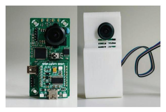
The SiliCam RIK is a fully programmable embeddable stereo camera, which provides simple vision capabilities to small-embedded systems in the form of an intelligent camera.
