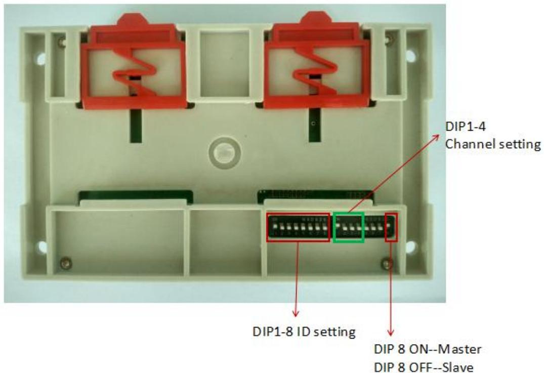
1) Outer(right side) DIP 1-4 are used for channel setting. Please check the following definition:
