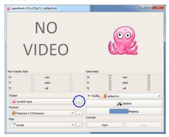
a. in the "Tracker" combo box, select "Joystick input", and click the button next to it, you will open a new window;
