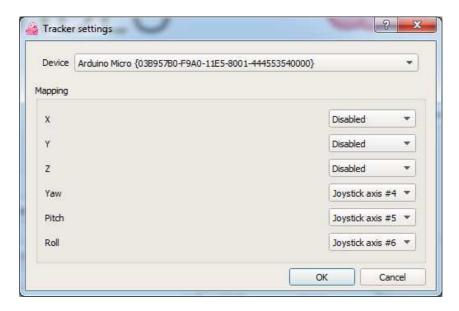
b. in Device combo box, select "Arduino Micro", and set the mapping as shown in the figure. Then, click OK to return to opentrack;
