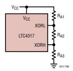
Figure 6. Address Translation Byte Configuration Using Three Resistors
