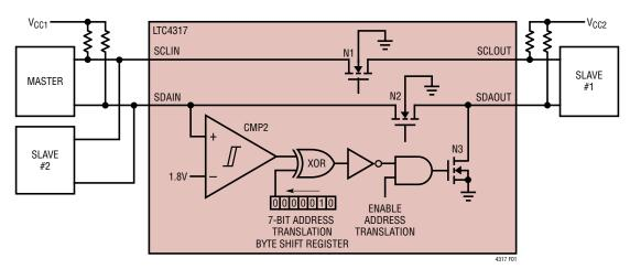
Figure 1. Basic Functions of the LTC4317
