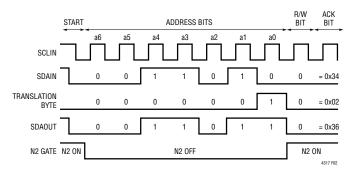
Figure 2. Basic Address Translation Waveforms
