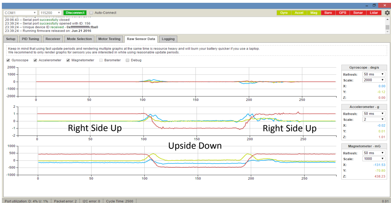
Figure 19. A time trace graph of the X, Y, and Z magnetometer signals showing that M_Z is symmetrical about the origin as the quadcopter is inverted. This indicates that the heading algorithm has converged to the correct state.
