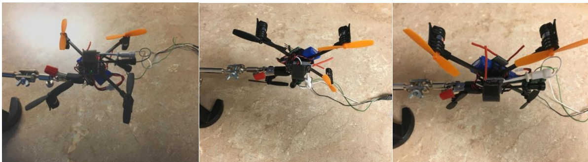
Figure 16. A U816 quadcopter held with each of the accelerometers aligned to gravity using an insulated "Third Hand" holding aid.
