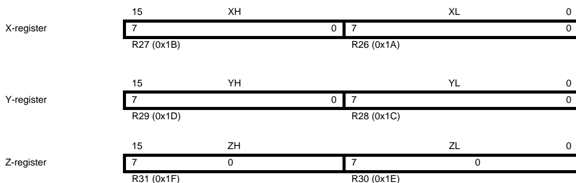
Figure 4-3. The X-, Y-, and Z-registers
