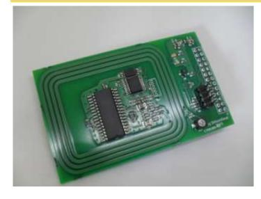
The NFC RFID reader for the Raspberry Pi is a complete read and write solution for the most common and widely used 13.56 MHz NFC cards and tags.
