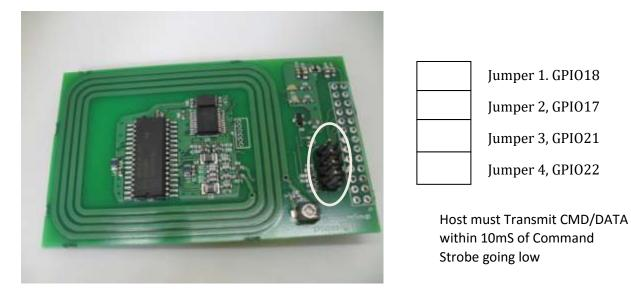
Only one jumper should be connected at any time. For example, connecting the jumper across the jumper 1 pins enables the Pi to select the Reader using GPIO18.
