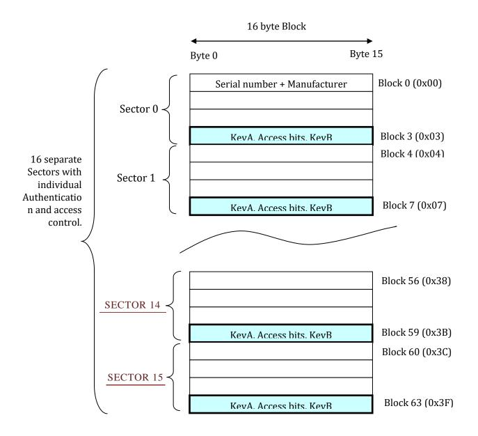
1024 byte memory is organised as sixteen sectors, each of which is made up of four blocks and each block is 16 bytes long. The first block in the memory (Block 0) is read-only and is set in the factory to contain the four-byte serial number (UID), check bytes and manufacturers data.
