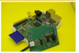
using the UART of the Pi for communication and the built in intelligence of the Reader the user is able to operate the reader without the need for libraries to be downloaded and compiled onto the Pi. The reader is intelligent and performs reading and writing of tags independently of the Pi. All of the tag read/write data is available to the Raspberry Pi.
