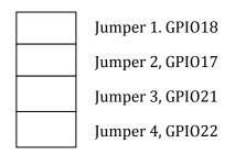
Only one jumper should be connected at any time. For example, connecting the jumper across the jumper 1 pins enables the Pi to select the Reader using GPIO18.
