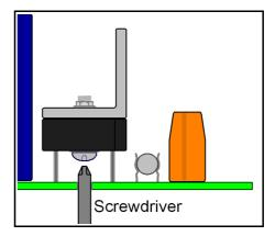
Wires may be soldered directly to the PCB, or you you can use screw terminals if you like. Direct soldering saves a few dollars and potentially increases reliability, as screw terminations may be prone to loosening in a high vibration/movement environment such as may be found on the road.
