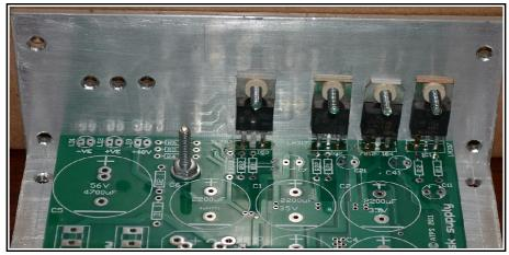
Remove the board from the case and finish assembly by next inserting all the smaller components such as the resistors and smaller capacitors – except for C13, leave C13 until later, also if you are unsure about using soft-start then leave out the soft start capacitors C4 and C24.
