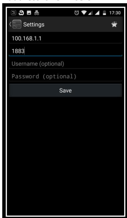
Figure 20: MQTT broker IP address and port number entered
