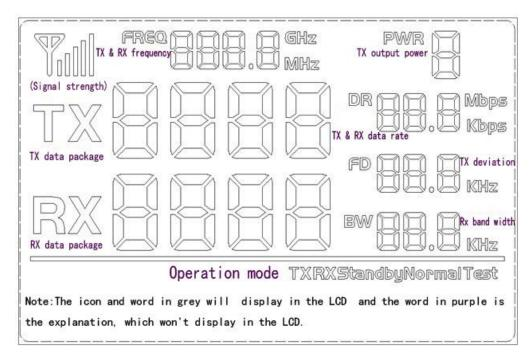
Users can set the parameters of the RF module such as frequency / transmitter power / transmission data rate / working mode through the buttons, and measure the wireless communication distance. Also, all the connection Pins of the module are extended to the demo board, user can use oscilloscope, multi-meter to monitor the operation of the RF module, which is very useful for software programming.
