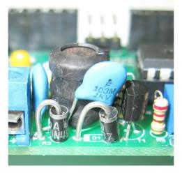
Then add external diode and capacitor. Load resistor should be installed on tube. This hardware mode adds voltage multiplier that allows to get 600V. Please modify PWM settings and upload new sketch before connecting multiplier! PWM values are experimental, start with 30 and increase it in small steps for getting 600V. Additional insulation required for external components! Use epoxy resin isolator or, at least, a heat shrink isolator.
