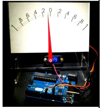
Shown connected to a standard Arduino with three breadboard jumper wires. Red for +5, black for ground, and orange is the PWM signal. That's it, a single digital output is all you need for a gauge.
