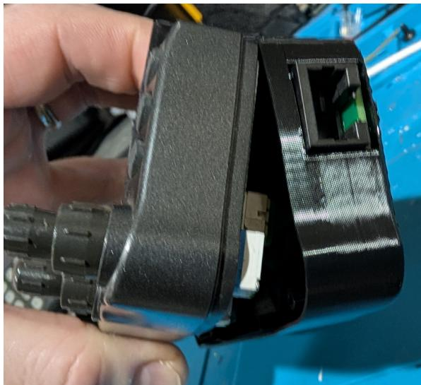
Hinge the cover over the front of the control head starting at the top clips and seating the bottom last. Use the screws you removed from the original cover to secure it. DO NOT OVERTIGHTEN!
