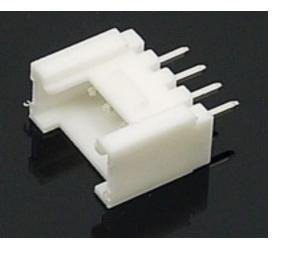
The way we have been wiring I2C connections before just didn't work for large projects. Basically, we used to put the I2C bus to screw terminals or snap down connectors and then ran wires to each device. This would not work for complex projects. Because of this, we moved to Grove connectors [http://www.seeedstudio.com/wiki/Grove\_System].
