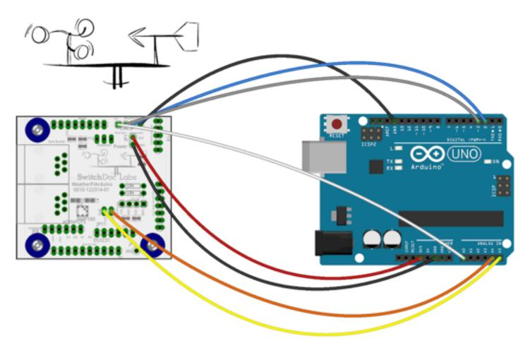
The Arduino contain an onboard 6 channel analog-to-digital (A/D) converter. The converter has 10 bit resolution, returning integers from 0 to 1024. The Arduino ADC does have some issues with accuracy and sample speed. If you have a long cable running to the WeatherRack sensors (Wind Vane especially), you will have issues reading the correct wind direction (as well as noise issues. If you have noise issues, bypass the Wind Vane line with 0.1uF bypass capacitors to ground.).
