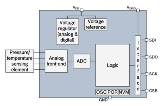
The BMP280 as shown above is a high precision I2C Barometer / Temperature sensor. Older WeatherPlus board (before revision 0011-021916-01) have the BMP180, the previous member of this family.
