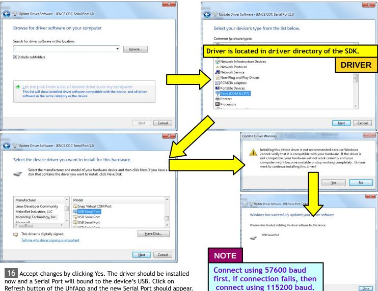
Refresh button of the UhfApp and the new Serial Port should appear. Connect to this Serial Port. Hit Scan to scan.
