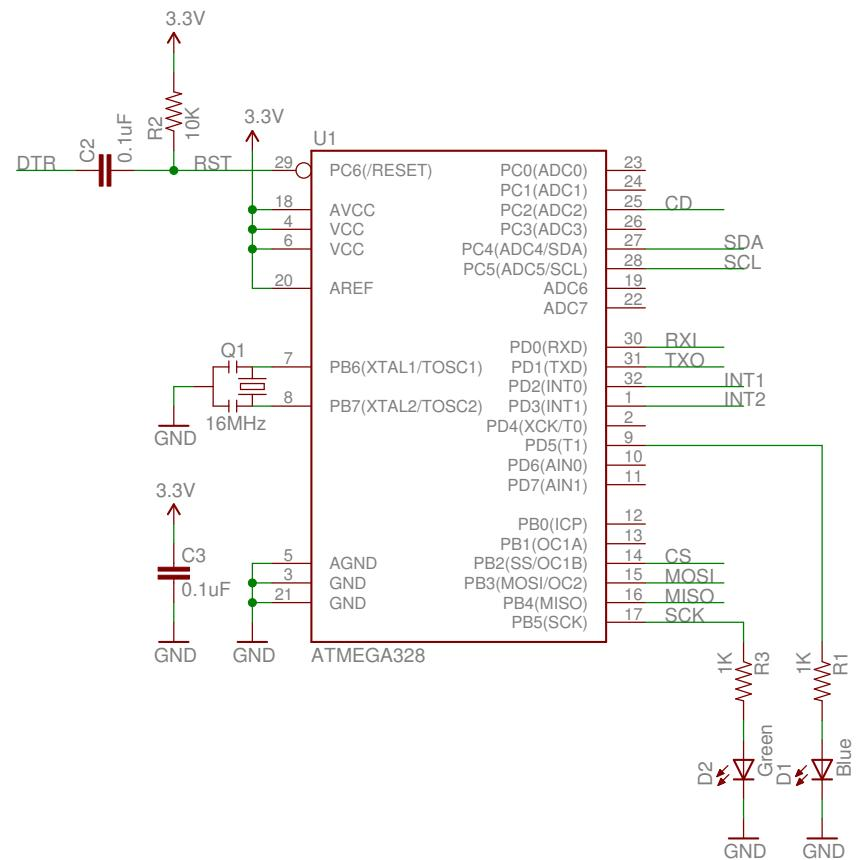
Remember, RXI is an input pin into OpenLog.
