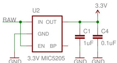
Max Voltage Input: 16VDC
