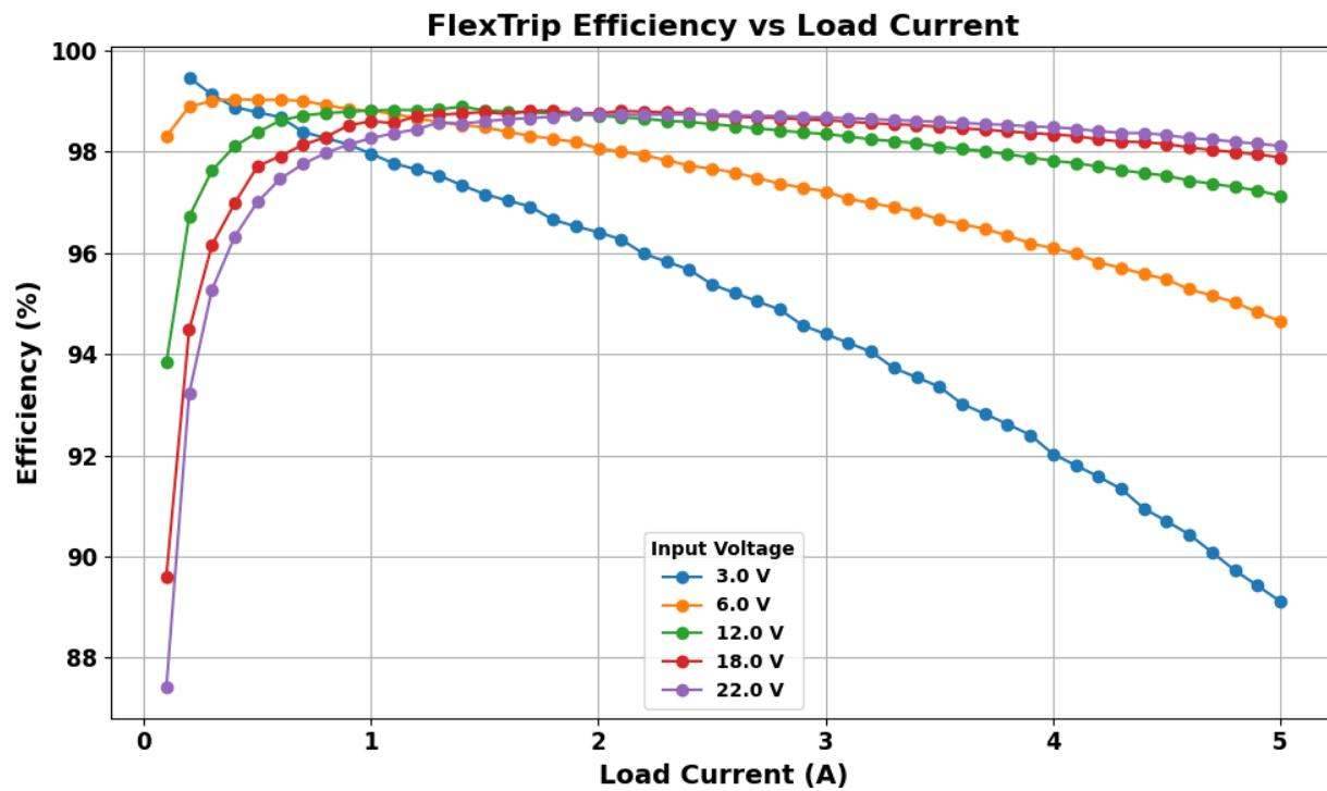
The efficiency was measured as a standard DC:DC converter. A 4-wire measurement of the output voltage on the electronic load was made, and the output of the power supply was compensated to account for the voltage drop in the wires going to the device.
