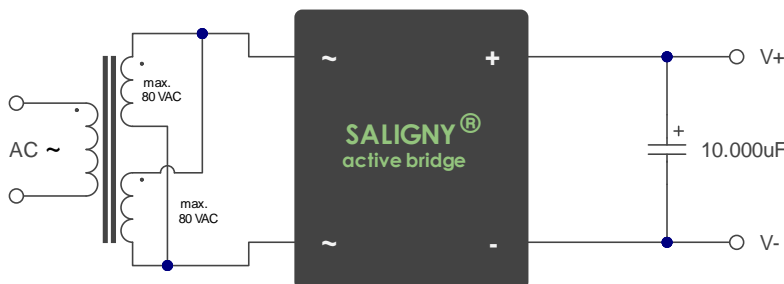
Fig. 7 - Full-wave rectification with dual identical secondary windings connected in parallel.
