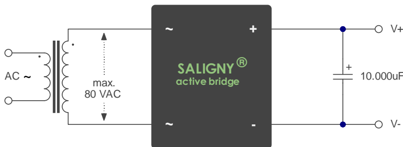
Fig. 6 - Full-wave rectification using a single secondary winding.
