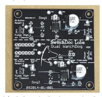
Why do you need a external Hardware WatchDog on an Arduino or Raspberry Pi? The reason is the internal watchdog is disabled in the bootloader for the Arduino and the Raspberry Pi is difficult to use and is not the same as rebooting by turning the power on and off (the internal Raspberry Pi Watchdog does not reset all peripherals).
