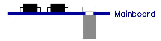
If building the keyboard with overlay, the spacer is placed between the keyboard and the overlay, and the screws go through these into the pillars.
