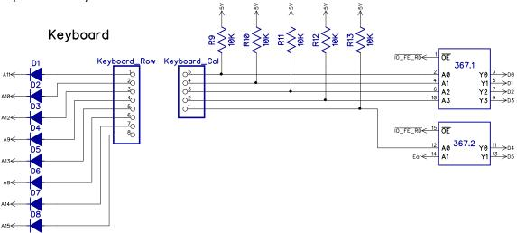
The keyboard is mapped as follows, this is very similar to the ZX80/ZX81, other than most of the bottom row is shifted one character to the right, at least logically. The Symbol Shift key is physically located between M and Space, but logically it sits between Shift and Z in the keyboard matrix.
