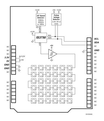
The core of the Kappa3750Ard is the IS3750 I2C Addressable LED controller chip, which is connected to a 5V Schmitt trigger. The Schmitt trigger converts the 3.3 V LED data output to 5 V LED. Generally, addressable LEDs operate at 5 V, so the Schmitt trigger matches the 3.3 V output of the IS3750 to the 5 V level required by the LEDs.
