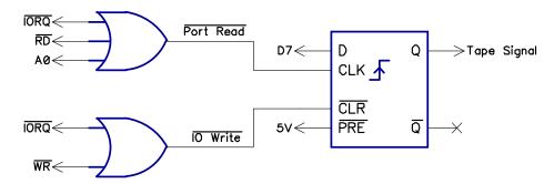
At this point, it samples D7, the data from the tape as the Z80 will see it, digital data, rather than the analogue tape input signal.
