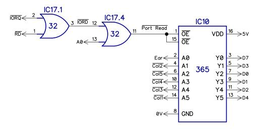
When the Z80 makes an IO read request and the address is even (A0 is low) the 74LS365 will place the inputs on the databus in time for the Z80 to read the bus on the rising edge of the IO request.
