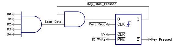
The Minstrel Input Monitor uses the second half of the flip flop to latch the scanned data on the port read.
