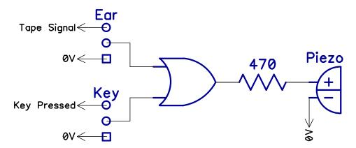
The OR gate mixes the signals to drive the piezo sounder.
