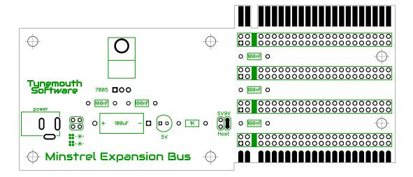
If the 9V jumper is not fitted, then both the host and the expansion bus need their own 9V power supplies to be connected.
