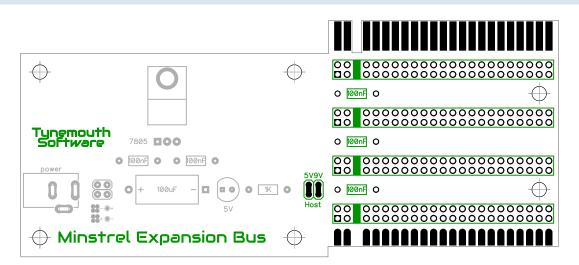
If none of the optional power parts are installed, then the 5V and 9V jumpers can be installed to power the 4 expansion slots and the edge connector from the host power. You could optionally add the 1K resistor and LED if you wish.
