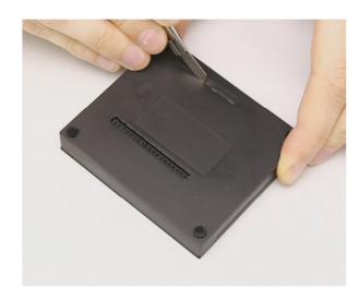
Using a sharp knife, cut little by little the slots located in the back of the Mooltipass.
