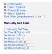
In situations where satellite signal is impossible, but you want devices on your network to have synchronized time. You can manually set time. Note: The device can drift as much as 45ms per hour.
