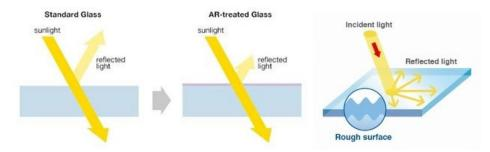
An LCD screen with external film solves this issue nicely. As for automotive applications, in an accident, broken LCD with top AR film won't produce sharp edge glass that could harms auto occupant. Nevertheless, a top film always reduces TFT LCD's surface hardness. And it is susceptible to scratches. On the other hand, AR coating retains LCD's hardness and touch performance. But it comes with a bigger price tag.
