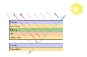
Putting any film on the top will reduce LCD's surface hardness, and polarizer will cause a loss in transmission. Those are not very ideal.
