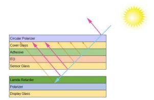
This method is very effective for an LCD display with resistive touch panel. We know resistive touch LCD has two air gaps: air gap between two ITO (Indium tin oxide) layers and air gap between touch panel and LCD display. Reflectance caused by the two air gaps is very high. Applying circular polarizer blocks off most of the reflected light, and makes the LCD display sunlight readable.
