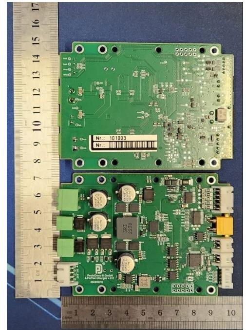
PDCharger module based on the newest STM32 microcontroller utilizing the power and cost-effectiveness of the latest industry standards. PDCharger could be customized for any type of battery.
