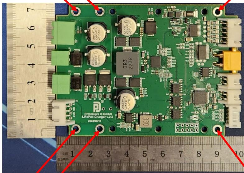
Mounting holes (d=3.2) for mechanical mounting with M3 screws.
