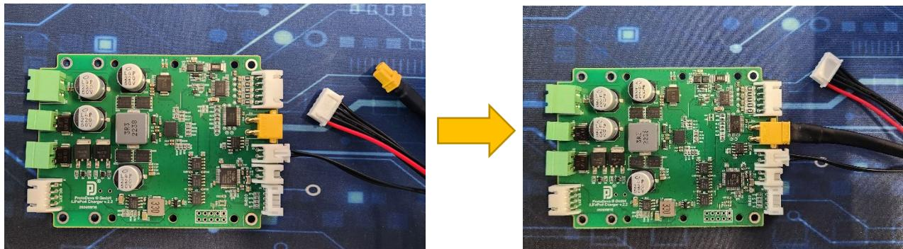
**Step 3:** Connect Battery balancer connector (5 pin, white -> to X42)
