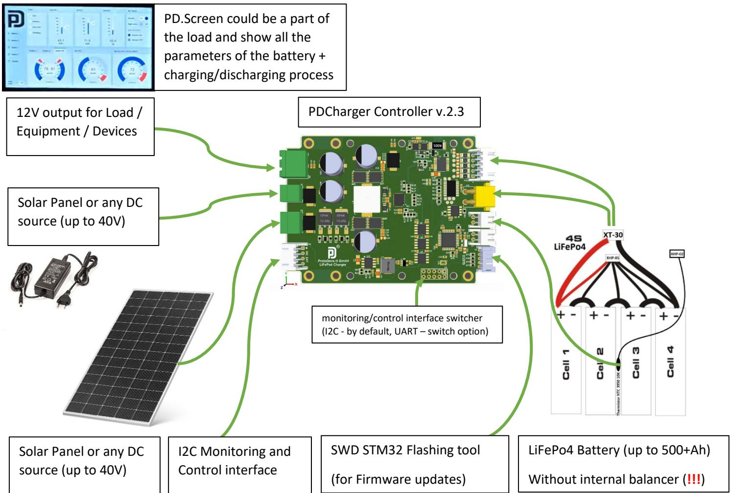
PDCharger Controller consists of 4 major blocks: [SMT32 MCU](#), [BMS chip](#), [Gauge chip](#) and [Charger chip](#).
