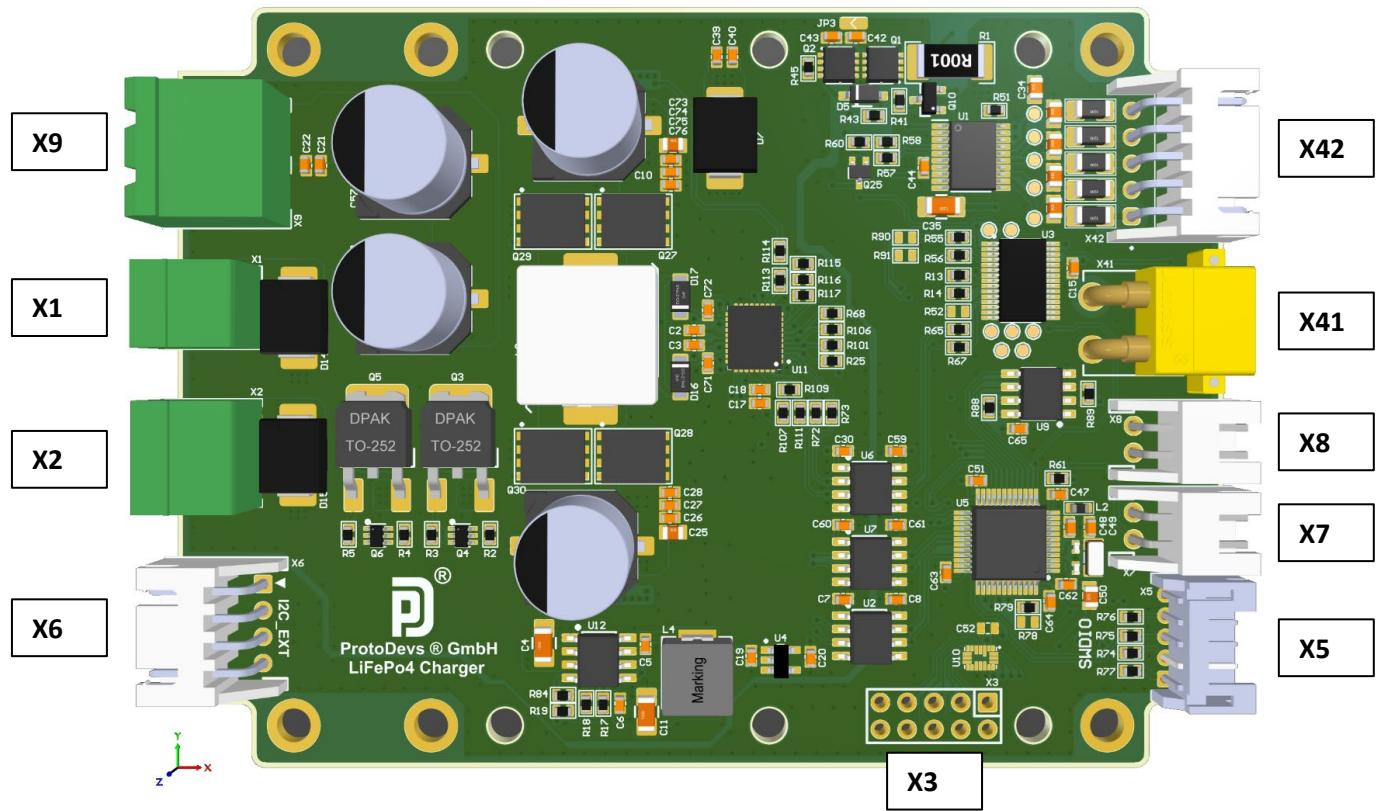
**X1:** Input, input #1 (3.6-V to 24-V wide input operating voltage) :
