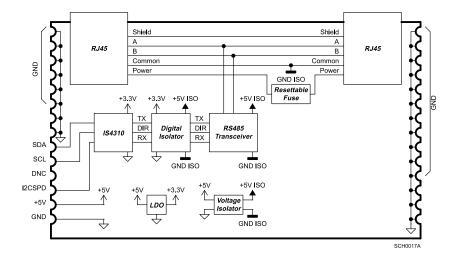
The IS4310-ISO485M6 is a compact ( $44 \times 28$  mm) module with castellated holes, designed for PCB mounting to function as an RS485 Modbus RTU Slave. It features two key components: the Modbus RTU Slave Stack (IS4310) and an RS485 transceiver.
