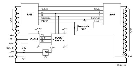
The IS4310-485M2 is a compact ( $44 \times 24$  mm) module with castellated holes, designed for PCB mounting to function as an RS485 Modbus RTU Slave. It features two key components: the Modbus Slave Stack (IS4310) and an RS485 transceiver.
