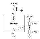
3. For a **1000MHz** setting, set the I2CSPD pin to VDD.
