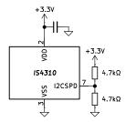
For a 1000MHz setting, set the I2CSPD pin to VDD.
