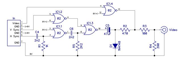
The video signal is active-low, so the white pixels are low, this is inverted by IC1.4.
