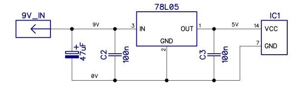
The board contains its own 5V regulator, to avoid noise on the video signals from the digital logic.
