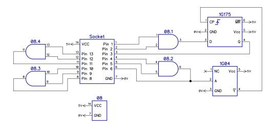
The flip flop is triggered on the rising edge of the clock, which is not ideal, so an inverter is added to invert the clock signal first.
