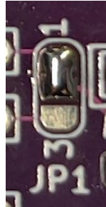
Step 2 Completed Bridge
