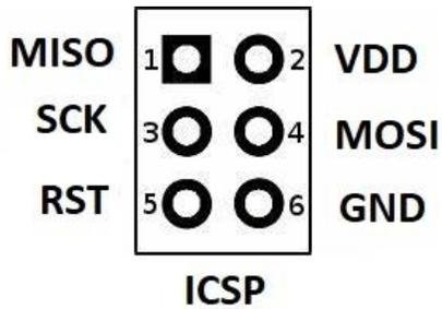
The ICSP connector follows this layout which is the same used for Arduino boards. There are a number of YouTube videos showing various methods for programming including using UNO or Nano boards as an AVR In System Programmer using the ArduinoISP sketch.
