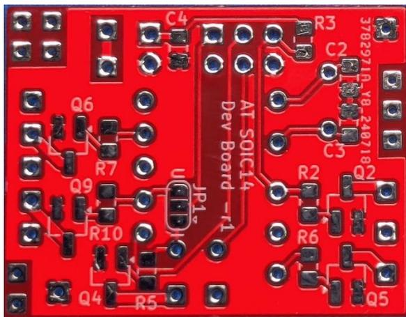
The AT SOIC14 development board supports a variety of 14 pin SMD parts with ICSP or UPDI programming options (See the Board Details for a list of devices). Generally, those parts in a SOIC14 narrow package with VDD at pin 1, GND at Pin 14, and UPDI on pin 10 or ICSP should work.
