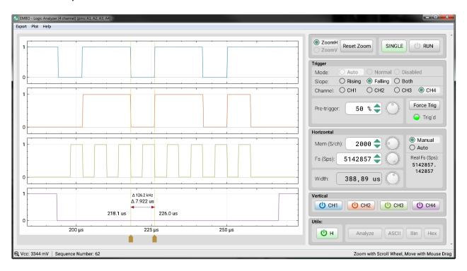
Most controls share the same functionality and design with the oscilloscope. The difference is with the trigger, where the trigger level is missing, on the contrary, the possibility to trigger on both edges (Both) has been added. Furthermore, the vertical gain and offset are missing because they do not make sense for the logic analyzer. Similarly, averaging mode, bit resolution, and FFT are also missing.
