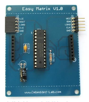
At the end, you need to install the LED matrix module. While doing so, make sure that the pin number of the matrix module goes into pin marked with 1 (with a circle) on the PCB. The pin number 1 of the matrix module is the first pin from left on the side where its model number is printed (see the pictures below).
