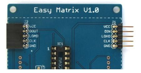
Next, install the two 8-pin female headers. Make sure they are aligned perfectly vertical. Again, do not solder all pins at once. After soldering one pin, check if it is going to be straight vertical.
