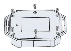
Step1: Remove the screws on the bottom of the device
