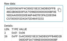
LEN. - length of EIR packet (Type + Data) in bytes, TYPE – the data type as in https://www.bluetooth.org /en-us/specification/assigned-numbers/generic-access -profile
