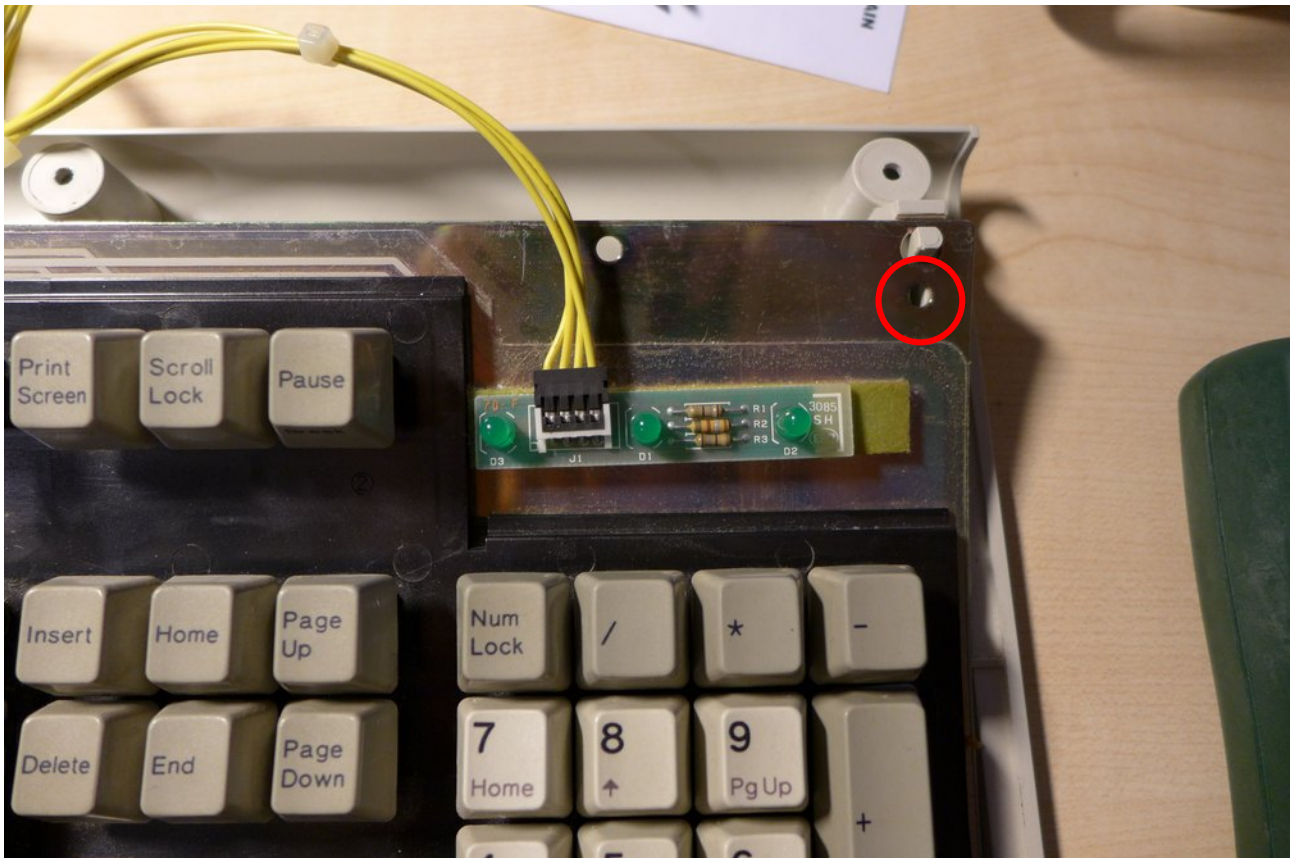
Open case with keyboard assembly and screw location (if present)
