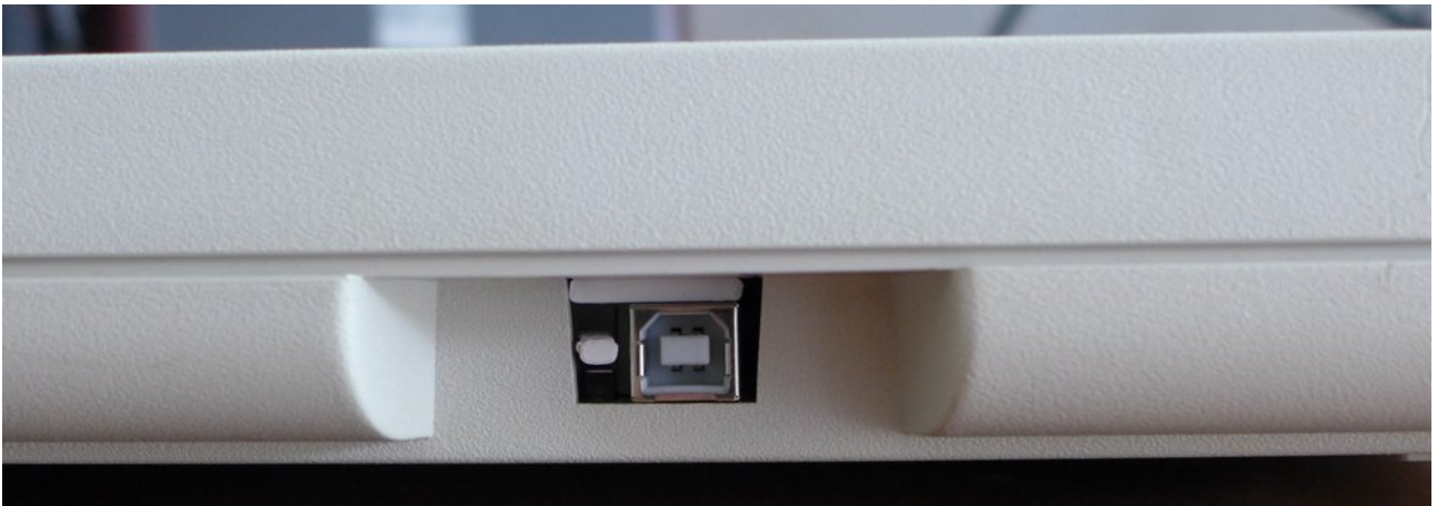
Finished assembly: Model M with USB port (visible as well the 3D printed spacer and button lever)
