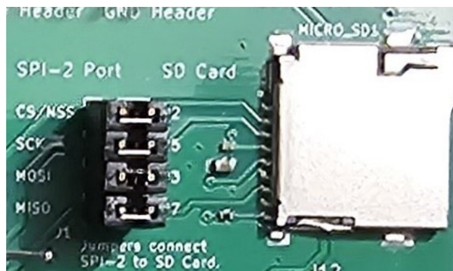
Figure 2: Jumper Setup for Micro SD via SPI-2
