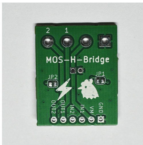
Figure 3: Rear side of the PCB of the MOS H-bridge.
