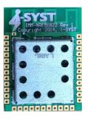
The nRF51822 is an ultra low power System on Chip (SoC) from Nordic Semiconductor. It integrates the nRF51 series 2.4GHz transceiver, a 32 bits ARM® Cortextm-M0 CPU, Flash memory, analog and digital I/O. The nRF51822 supports both Bluetooth Low Energy and proprietary protocols.
