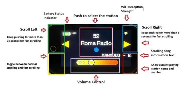
The radio is operated by one cell of 18650 3.7V Lithium- Ion rechargeable battery. For charging the battery you can use a standard phone type USB2.0 (USB A-USB C) 5V charging cable & charger.
