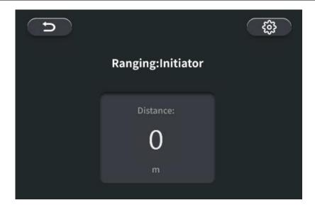
For example, as the initiator, the 'Distance' box will display the current distance to the responder. If the distance value is not updated within 3 seconds, it indicates a failure in data reception and the ranging process cannot be completed. In this case, three question marks '???' will be displayed in the 'Distance' box.
