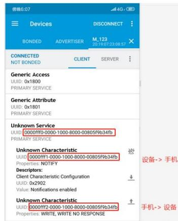
FFF0 is the service UUID, FFF1 is the cell phone receives data and the module sends data; FFF2 is the cell phone sends data and the module receives data.
