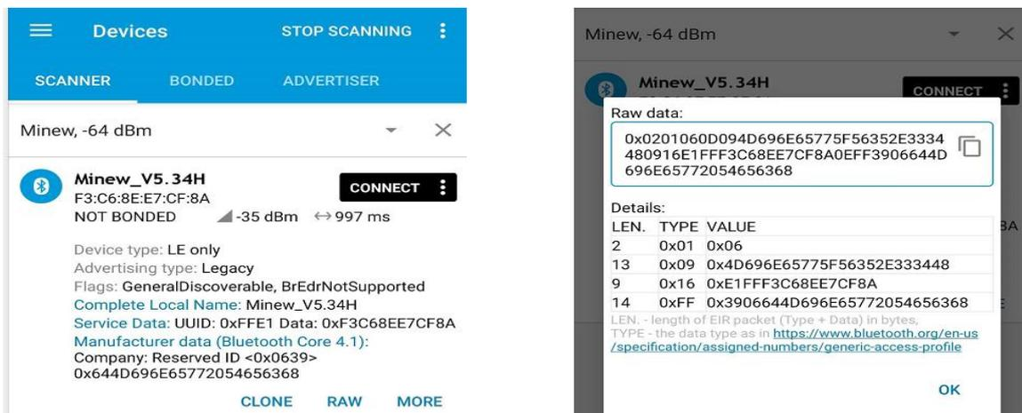
**Note:** The IOS side can not get the content of the MAC address field, so the MAC address is put back into the broadcast packet to ensure that the IOS side can get the device MAC address. In addition, the WeChat applet can't get the reply packet, so the MAC is put into the service data of the broadcast packet to ensure that the IOS side can also get the device MAC address using the WeChat applet connection.
