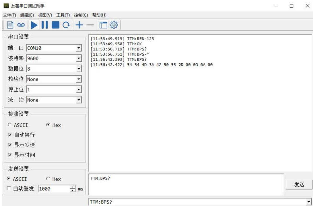
When querying the device parameters, because the parameters are hexadecimal numbers, when selecting the ASCII display, the parameter position may be garbled, at this time, you need to set to HEX display, the parameters correspond to the position after 2D, see the above figure, query the baud rate, you need to use the HEX display to view the specific parameters.
